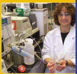
fthimia Papastavros, a graduate student in the lab of Dr. Hage, Chemistry, UNL, works with one of the highperformance liquid chromatography columns that the Hage lab is developing in partnership with Teledyne Isco. This column contains an immobilized protein for use in the selective extraction of drugs, estrogen mimics and other emerging contaminants from water.
