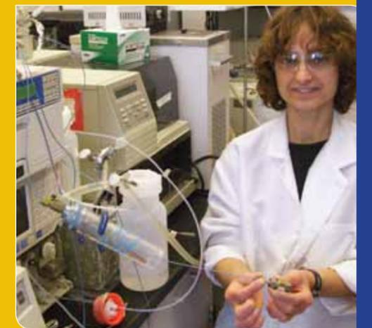
Efthimia Papastavros, a graduate student in the lab of Dr. Hage, Chemistry, UNL, works with one of the high-performance liquid chromatography columns that the Hage lab is developing in partnership with Teledyne Isco. This column contains an immobilized protein for use in the selective extraction of drugs, estrogen mimics and other emerging contaminants from water.
