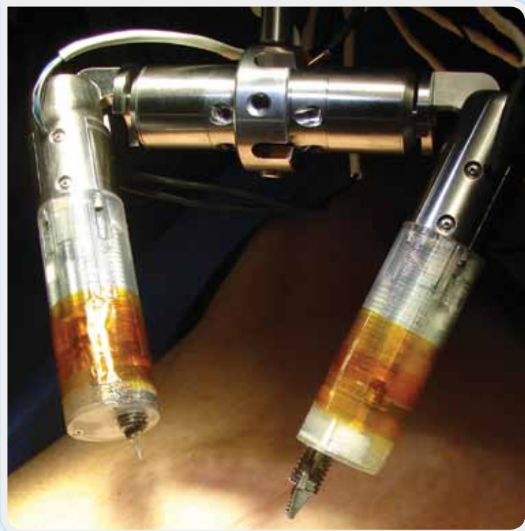
Miniature robots, such as this one developed by UNL's Shane Farritor, can help make surgeries minimally-invasive and more successful on long-duration NASA missions as well as in hospitals near you.
