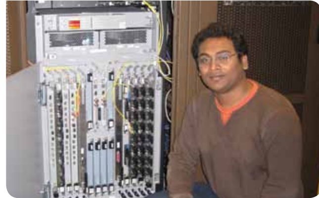
UNL/CSE graduate student, Praga Angu (supervised by Prof. Byrav Ramamurthy, UNL/CSE) posing in front of the Ciena CoreDirector (CDCI) optical switch deployed at UNL campus. The CDCI switch enables high-speed bandwidth-on-demand services which are vital for emerging eScience applications of interest to DOE scientists and university collaborators.
