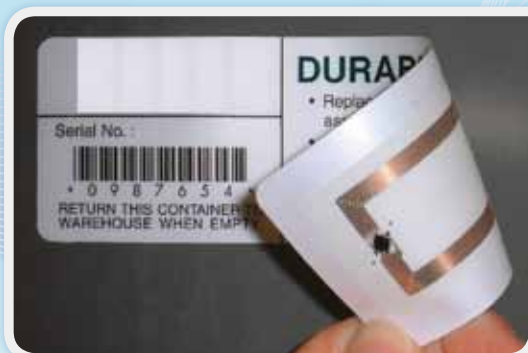
At left, a Radio Frequency Identification (RFID) tag could help NASA mission inventories.
